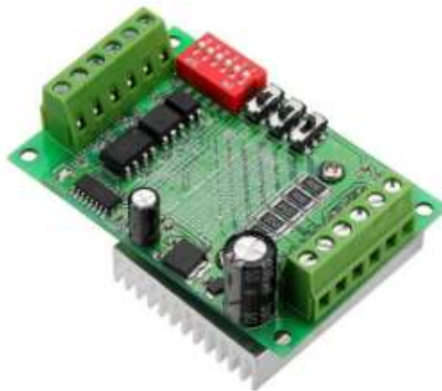
Figura 34. Driver motor a pasos TB6560.
