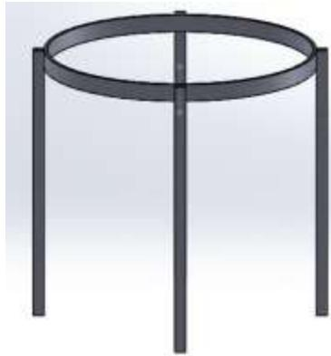
**Figura 35.** Base del reactor.
