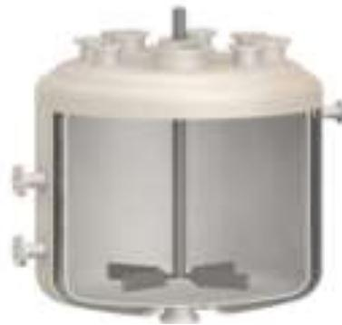
**Figura 16.** Reactor Batch.
