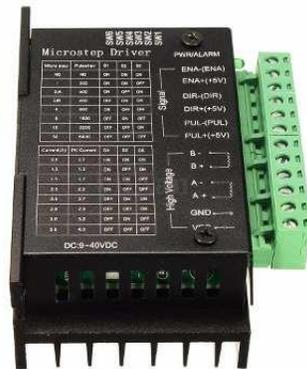
Figura 11 Driver Motor A Pasos Nema 23 4a Tb67s109a
